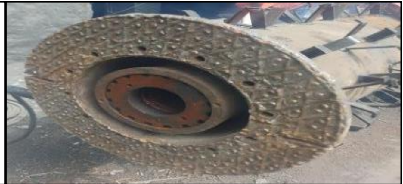
Tip Ring Hard facing done to enhance life
