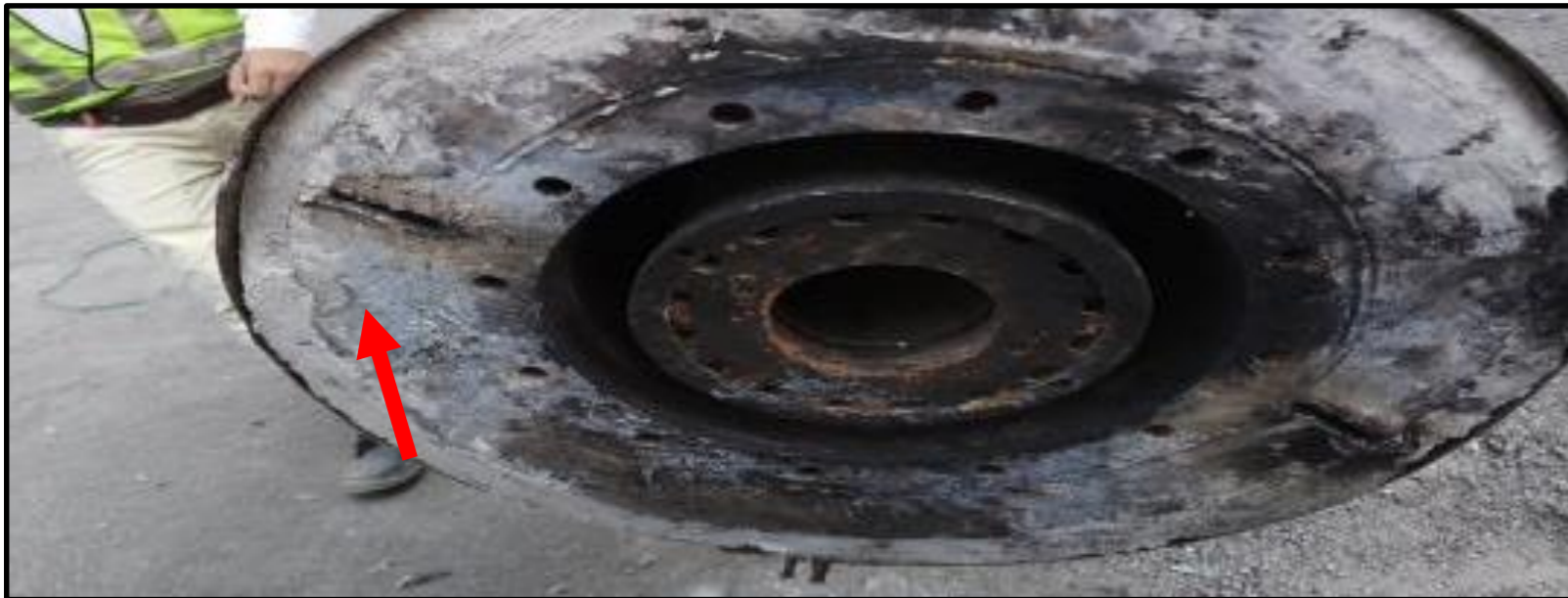
Burner pipe Tip ring & expansion gap provided to enhance refractory life KILN-3 BURNER PIPE
